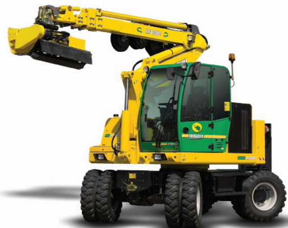
Typical flail-head tractor used for hedge maintenance.
